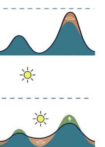
The EV battery thus becomes multi-functional – powering both the car and the energy network. Typically, a single car connected to the charging station can feed 10 kW to 20 kW of power back into the grid - enough to power several households at the same time.
